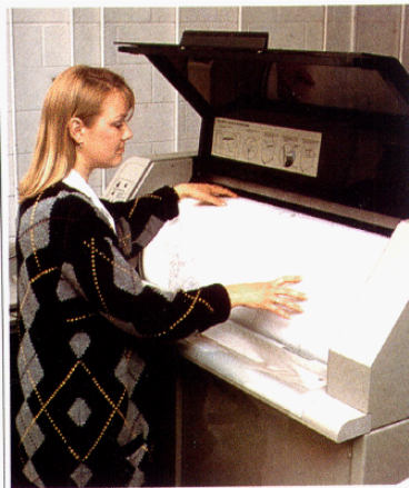
Figure 8. An electronic scanning device will convert some types of map information to digital form.
